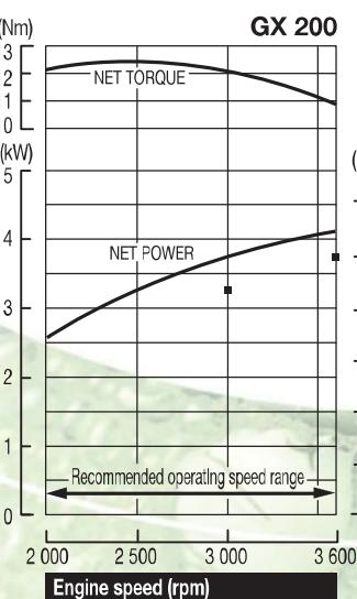
The power rating of the engine indicated in this document is the net power tested on a production engine for the engine model and measured in accordance with SAE J1349 at a specified rpm. Mass production engines may vary from this value. Actual power output for the engine installed in the final machine will vary depending on numerous factors, including the operating speed of the engine in application, environmental conditions, maintenance, and other variables.
